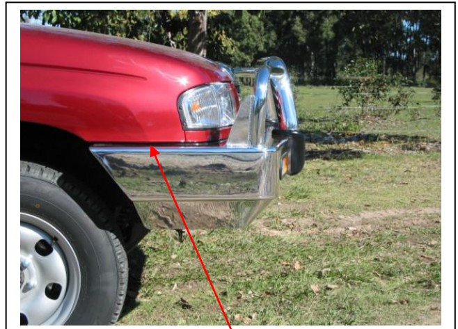
Figure 12 – Approx 12mm –18mm clearance
